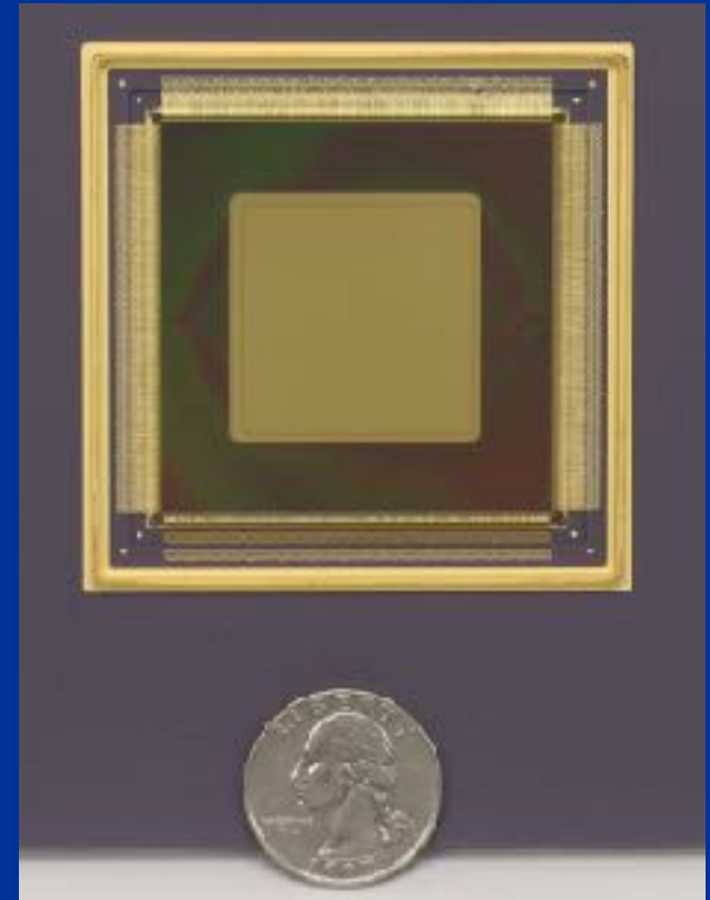
4096-actuator MEMS deformable mirror. Photo courtesy of Steven Cornelissen, Boston Micromachines
